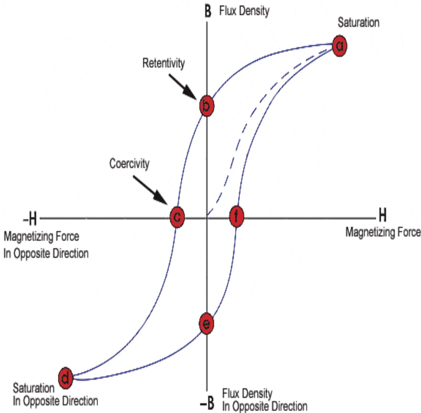
*Remanence*: a measure of the remaining magnetization when the driving field is dropped to zero.
